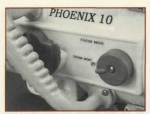
The magnetic switches on the left side of the housing control focus and zoom.
